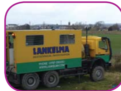
Truck mounted CPT Probing
